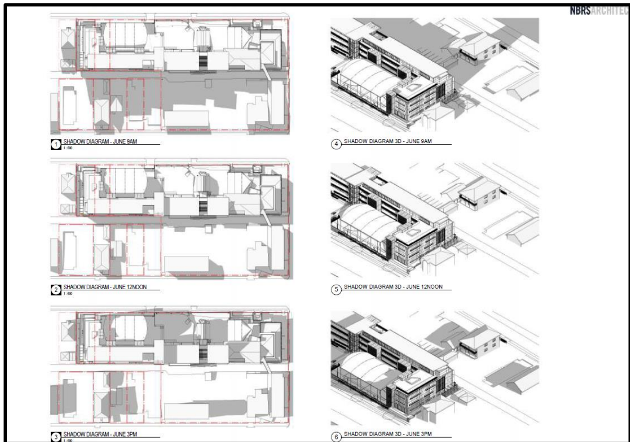
Figure 13: Shadow Diagrams showing that the proposed shadowing created by the development is compliant with the standards and every immediately adjoining property receives a minimum of 3 hours of solar access during the day in midwinter (courtesy NPBS 2017)
