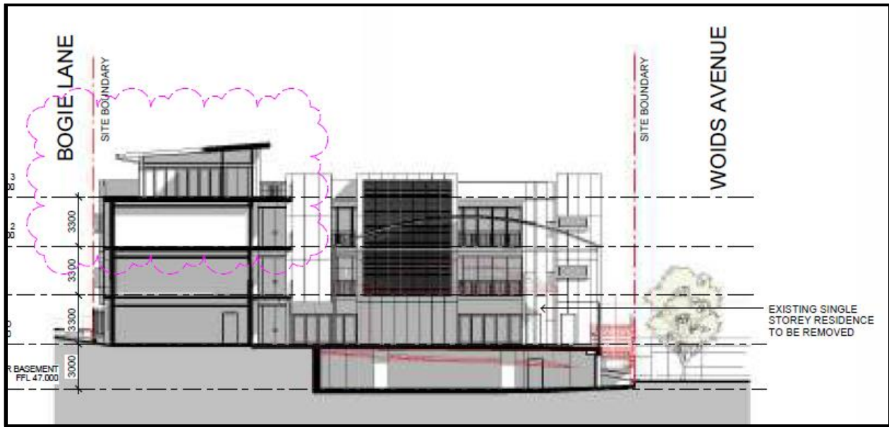
Figure 7: Short section of the building showing the point where the basement protrudes above the existing ground level towards the Woids Avenue Allawah frontage
